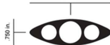
**FRAMES:** Base legs are made from quality 3/4" x 2" x .065 aluminum extrusion, Tig-Weld at all connecting points.
