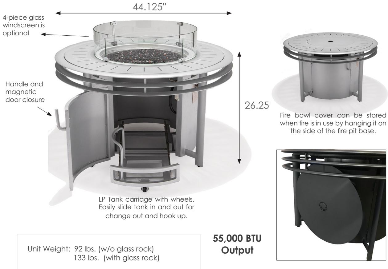
**FRAME:** Base legs are made from quality 3/4" x 2" x .065 aluminum extrusion, Tig-Weld at all connecting points. Top and side created from solid sheets of 3/16" aluminum stamped and/or formed.
