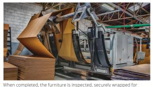
protection and placed into a heavy duty corrugated box for shipping. A newly installed box making machine makes boxes custom sized for each piece of furniture. A process that only takes seconds to complete.
