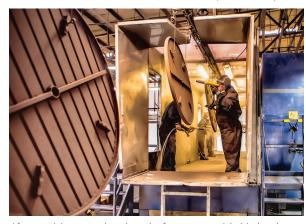
After receiving several washes, the frames are quick dried and enter the powder coating booths. The thick coating of polyester powder covers the raw aluminum with an extremely durable, protective finish coat.
