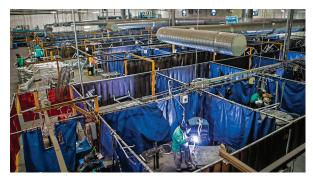
A host of machines that cut and bend the extrusions go to work forming the frames. Stacks upon stacks of cut extrusions make their way to the welding room where any one of 59 welding booths awaits the delivery.
