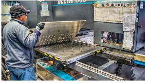
Other departments in the factory are creating furniture components. Some of which include the aluminum stamping machine. This device takes blank aluminum sheets that are placed underneath a die that punches out patterns and shapes for our stamped table tops.
